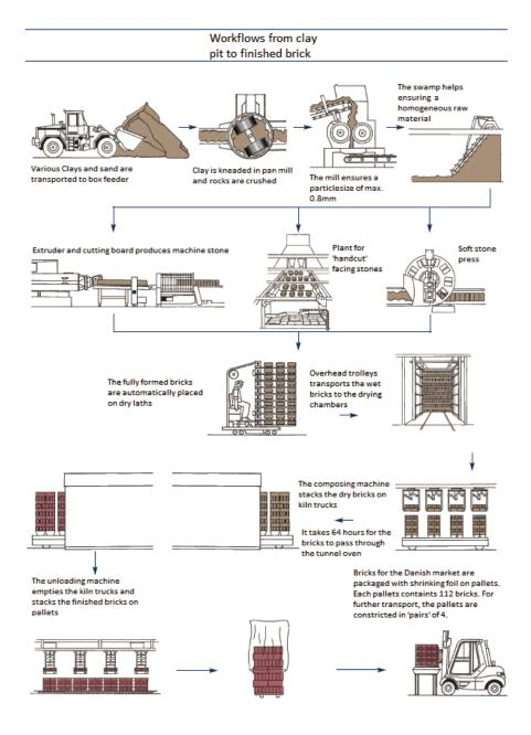
The flow diagram conforms with the requirements in the modular approach and shows the production phase A3 for brick production (Vesterled Teglværk only uses "soft stone press", no "extruder" and no "handcut"). The remaining phases are described below.
