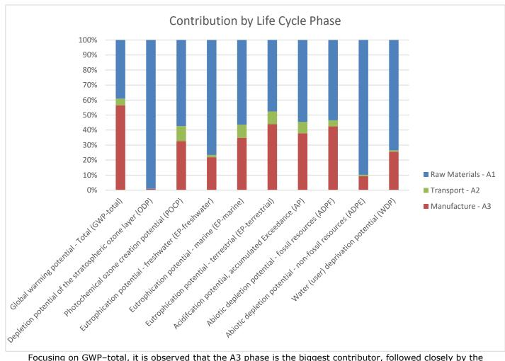
Focusing on GWP-total, it is observed that the A3 phase is the biggest contributor, followed closely by the A1 phase. The primary contributors across the phases are electricity use (40%), production of plastic granulate (16.7%), and waste incineration (11.5%). Other noteworthy contributors include the production of epoxy resins (10.2%) and potassium carbonate (3.8%).
