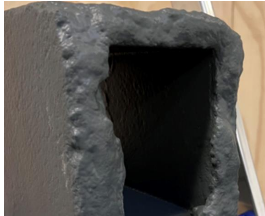
Figure 2 - Declared product, VC50, applied on ventilation duct of concrete.
