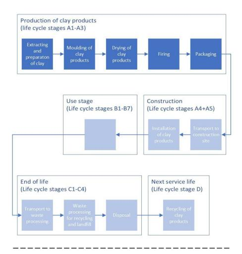
The flow diagram conforms with the requirements in the modular approach and shows the different stages.
