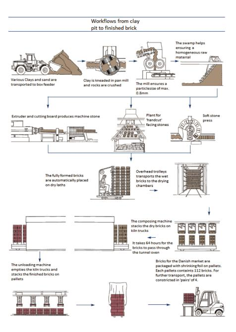
The flow diagram conforms with the requirements in the modular approach and shows the production phase A3 for Gandrup Teglværk with the exception that "handcut" is not used. The remaining phases are described below.
